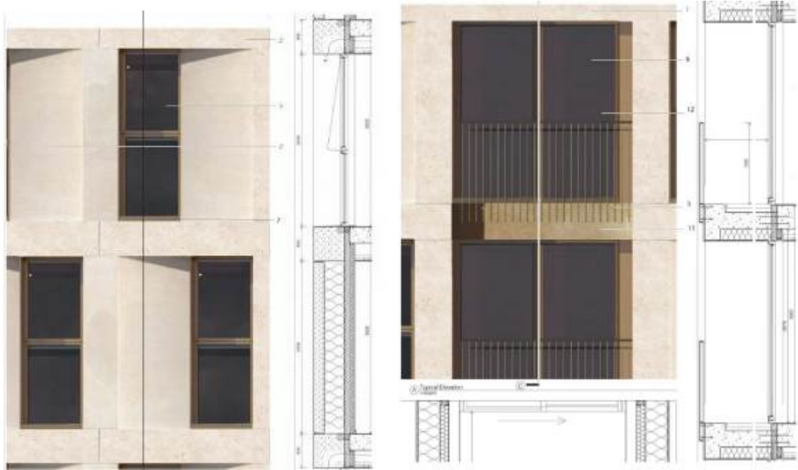
Bay study main façade
